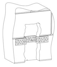
**2** Use the clamping system illustrated in the figure to attach the insulated pipe bend and screw on the nuts.
